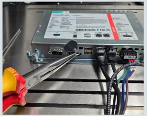
6. Place a new battery into the empty slot. Make sure the battery polarity is correct.
