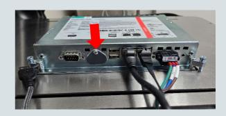
5. Remove the battery by GENTLY inserting a thin, small screwdriver (I used a terminal screwdriver) between the top of the battery and the HMI casing and lifting the screwdriver a small amount to push out the battery. This can be done 2-3 times until enough of the battery is sticking out that it can be grabbed with your fingers or needle-nose pliers.
