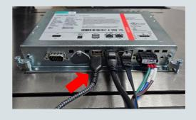
4. Using a T10 star/torx screwdriver, loosen the screw on the gray triangle cover (next to the USB terminals).
