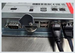
7. Put the gray cover back in place and screw down to secure. Plug the USB back into terminal x105 on the HMI.
