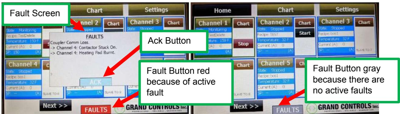
Figure 21: Faults screen and fault button colors
