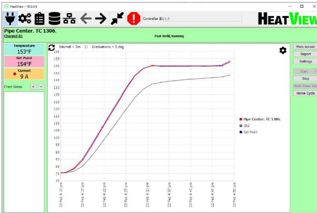
Figure 56: Master slave channels on enlarged chart.
