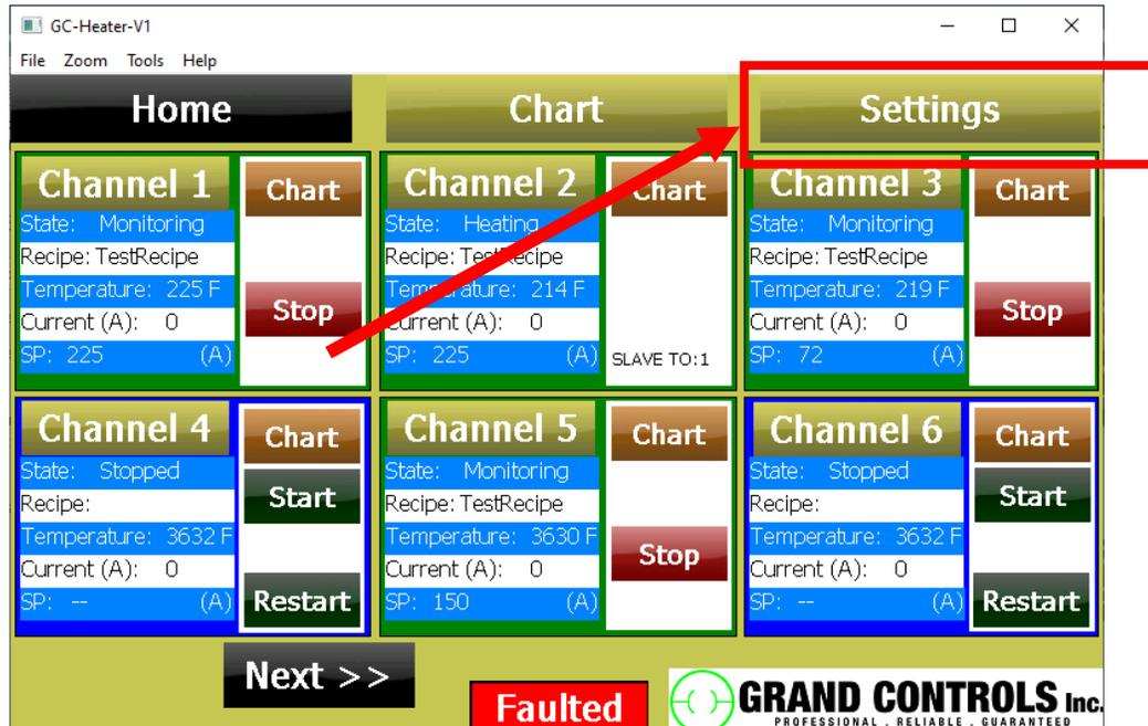
Figure 33: Selecting settings on the controller interface screen.
